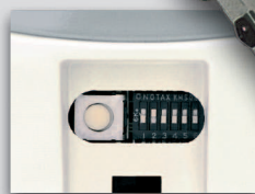
fig. 3: DIP switches for operator settings, such as up-date rates, memory mode, etc.
