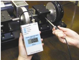
Stick the hand-held sensor to the measured object for measurement.
