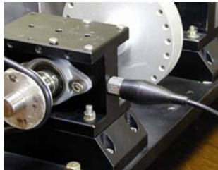
The sensor can also be screwed in position.
